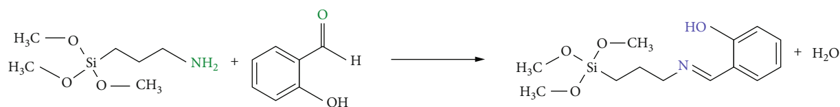
FIGURE 2: Schematic representation of the HSPTMS formation reaction. Proposed groups responsible for cation adsorption are presented in blue, and the groups that take part in the reaction are shown in green.
